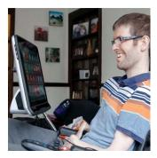
Eye tracking and eye control is a technology that makes it possible for computers to know exactly where the user is looking. When eye tracking and eye control are combined with speech generating devices and other opportunities.
